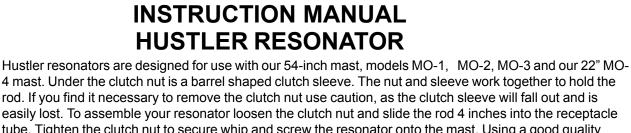
easily lost. To assemble your resonator loosen the clutch nut and slide the rod 4 inches into the receptacle tube. Tighten the clutch nut to secure whip and screw the resonator onto the mast. Using a good quality V.S.W.R meter check the resonate frequency. If it is too low, loosen the clutch nut and push the tip rod into the tube in ¼ inch increments until the desired frequency is reached. To lower the resonate frequency extend the rod in ¼ inch increments.
